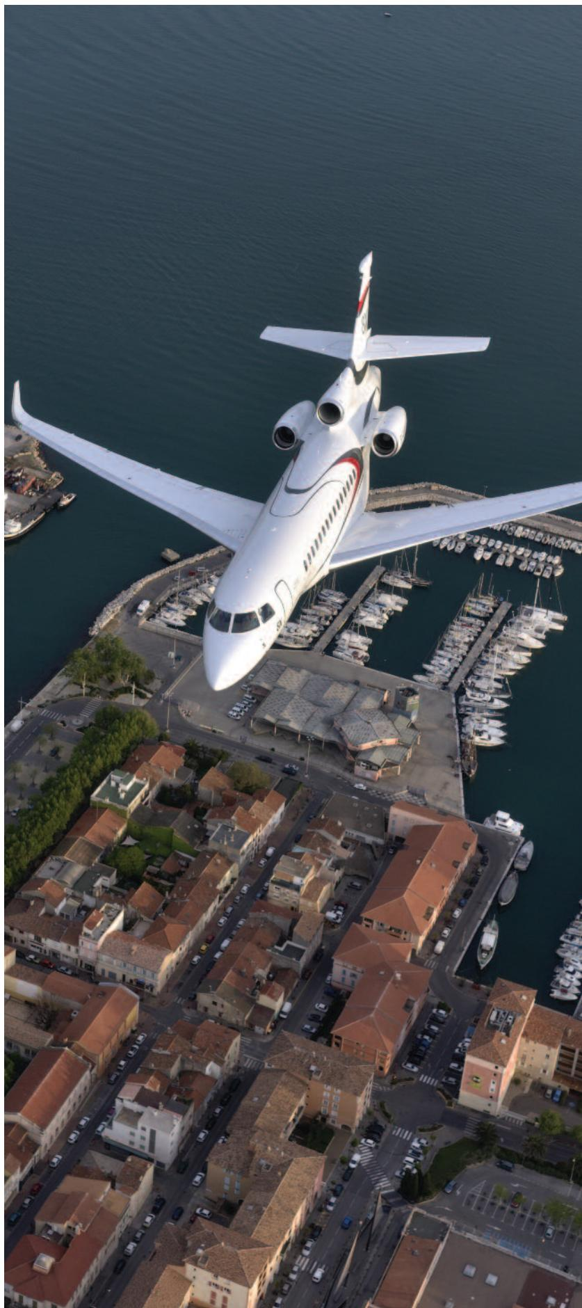
► Aviation derived the development of the Falcon 8X based on the 7X. The Falcon 8X is effectively an “ultra long-range” version of the 7X. While the exterior of the aircraft is very similar, the Falcon 8X features an extended fuselage, as the manufacturer integrated two additional fuselage sections to the front and back of the central section resulting in a cabin length of 13 m.
